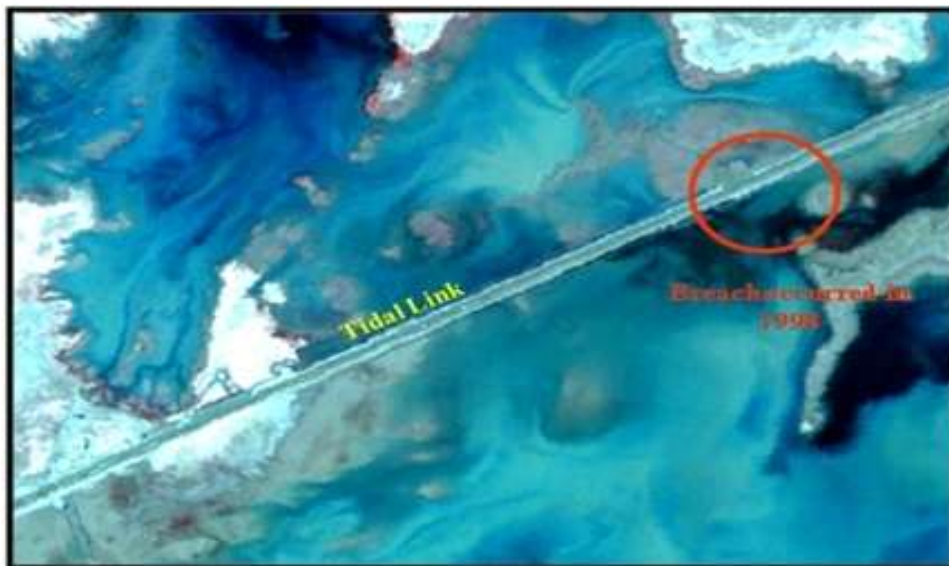
Figure 4: First breach occurred just after the construction of the Tidal Link Drain
